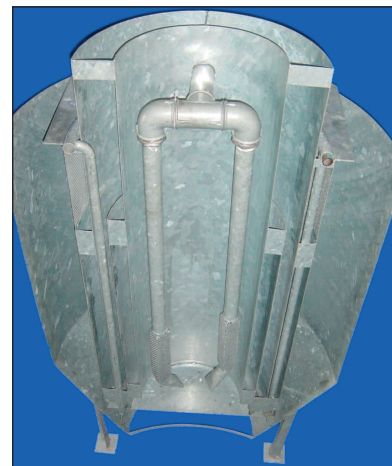
Section plane of the patented dissolution equipment
