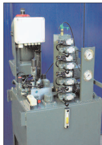
The hydraulic unit, manual and emergency for salt discharge
